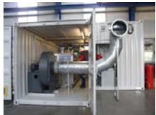
Adsorption system with catalytic oxidation, 6.000 Nm 3 /h
